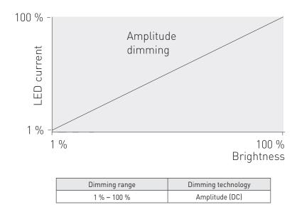
LL80DS-DA/AN-350-1400 LED driver implements amplitude dimming technology across whole dimming range. Amplitude dimming offers the best available technology for dimming the light output in an accurate and flicker-free way to ensure high quality lighting in even the most demanding situations such as camera recording applications. Amplitude dimming technology complies with IEEE 1789-2015 recommendations of current modulation to mitigate health risks to viewers.
