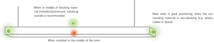
When installed in the middle of the luminaire and inside, the radio performance is poor if non-blocking material is not close.
