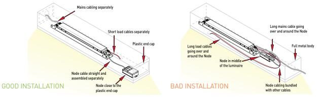
When the Freedom Node is installed inside luminaire with the driver, the following things needs to be taken in consideration regarding the communication:
