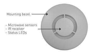
Microwave sensor: Detects movement within the detection range allowing load control in response to changes in room occupancy. IR Receiver: Receives control and programming commands from a Helvar infrared remote handset (available separately). Status LED: The red LED flashes to indicate the following:
