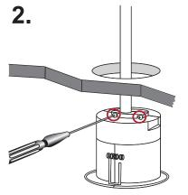
Attach the cable clamp.
